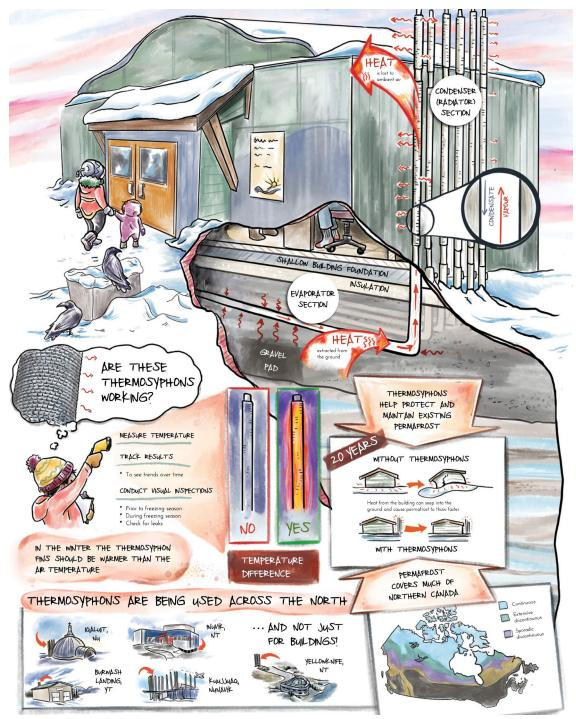
Figure 6.11: Infographic illustrating how thermosiphon foundation systems function, which ultimately aim to stop heat from a building from damaging the permafrost located beneath it. Source: Standards Council of Canada, 2020b.
