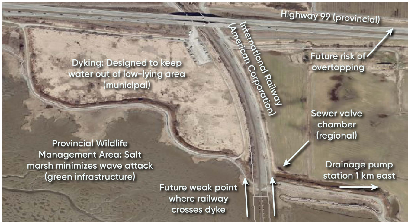
Figure 7.15: Interconnected infrastructure in Mud Bay, Surrey, BC highlighting the need for coordinated approaches in addressing risks presented by sea-level rise and other hazards. Source: Adapted from the City of Surrey, 2018.
