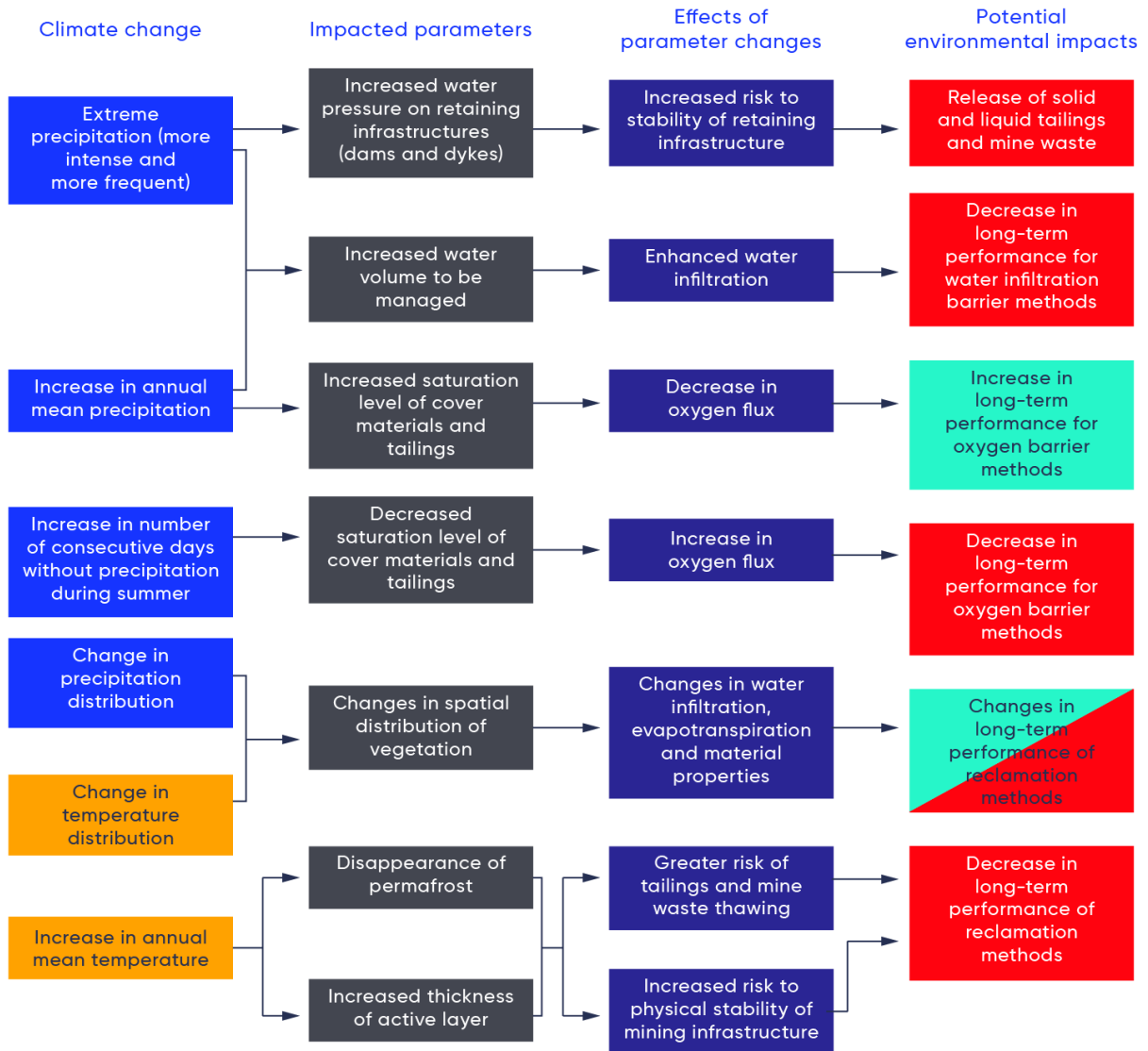
Figure 7.11: Summary of expected major climate changes and their implications for mine waste containment and reclamation structures.
